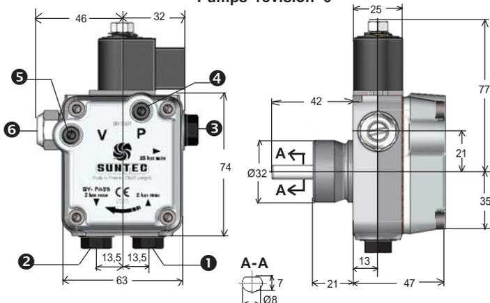
Inlet ① and Return ② with direct sealing for revision 6 models (sealing with washers can also be used)
