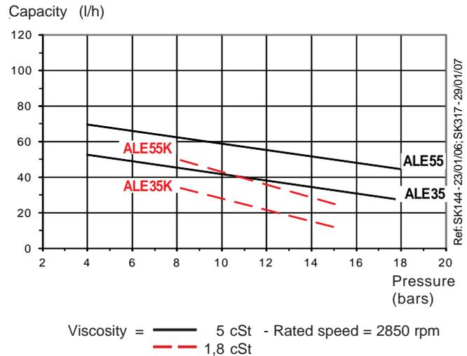
Data shown take into account a wear margin. Do not oversize the pump when selecting the gear capacity.
